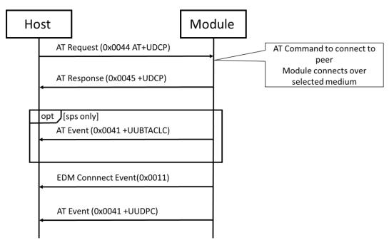
Figure 2: Connection setup
