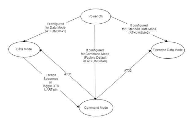
Figure 1: State diagram of the different modes for the module
