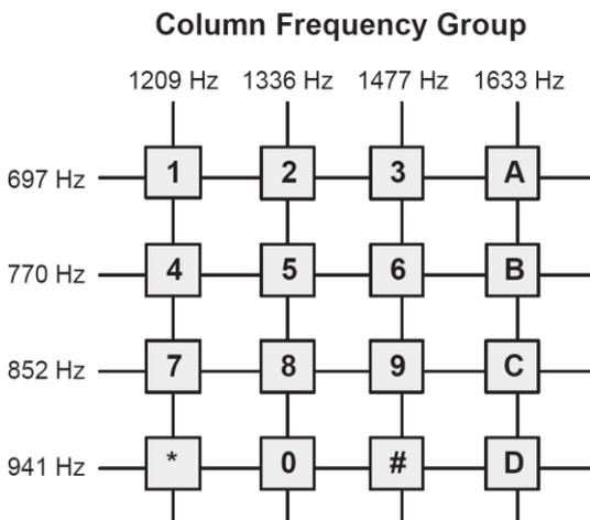
Figure 3: Touch-Tone telephone keypad: a row and a column tone is associated with each digit
