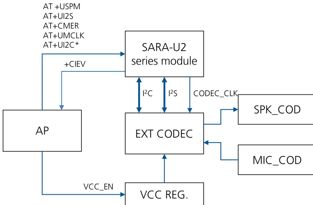
**Figure 2: External codec management for SARA-U series module**
