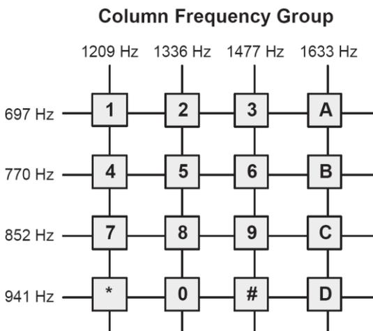
Figure 4: Touch-Tone telephone keypad: a row and a column tone is associated with each digit
