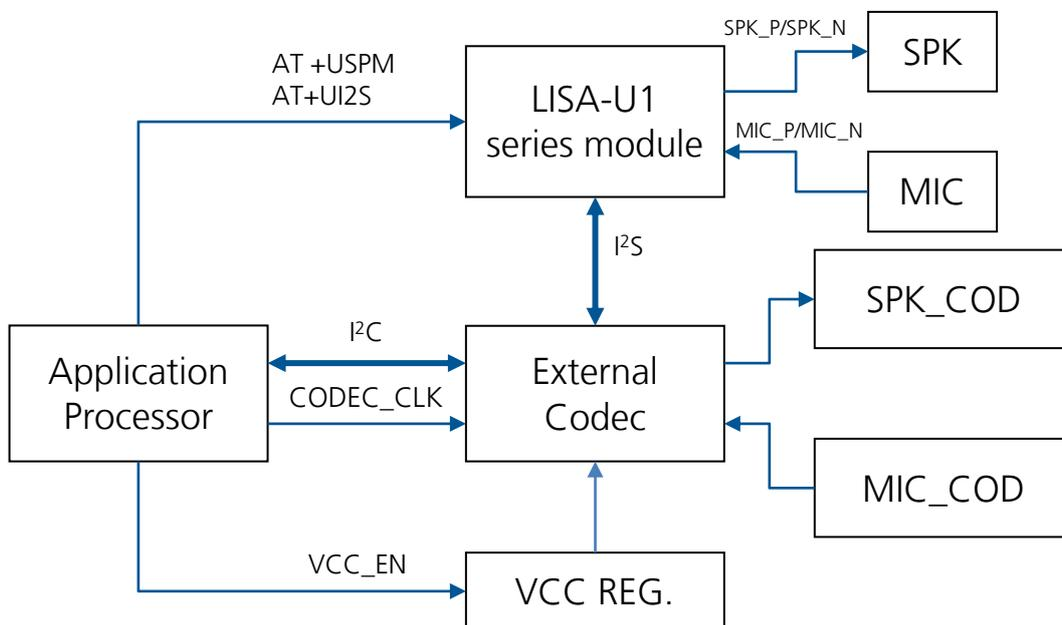
Figure 2: External codec management for LISA-U1 series module
