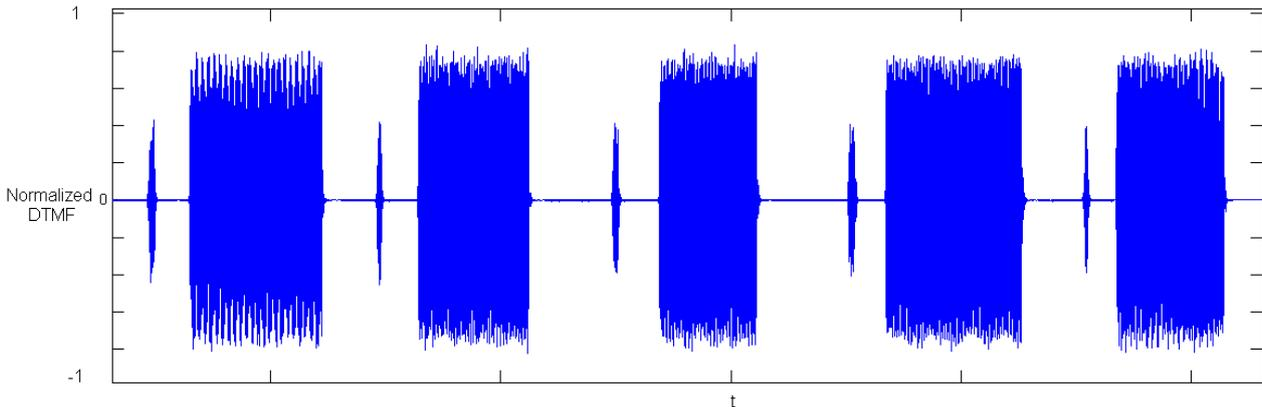
Figure 5: Normalized tones corresponding to digit presses '1','2','3','4','5', with interruptions caused by VoIP-based connection
