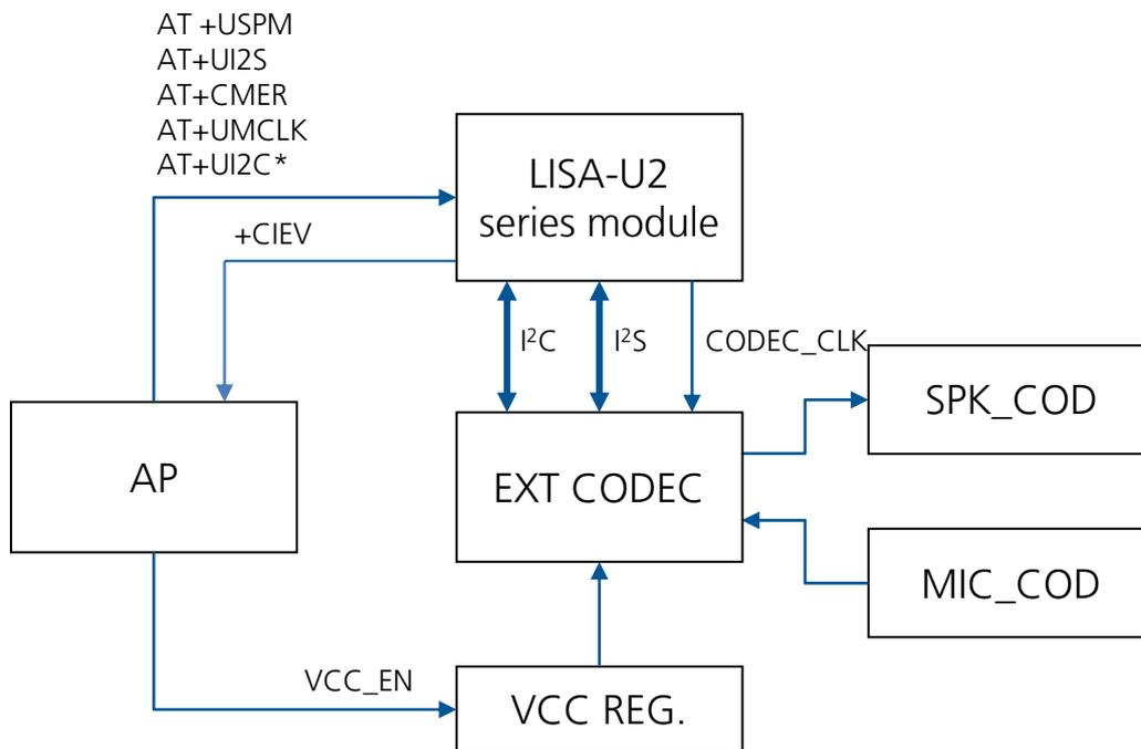
**Figure 3: External codec management for LISA-U2 series module**
