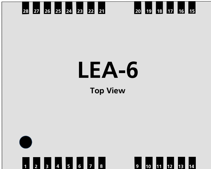
Figure 2 LEA-6 Pin Assignment
