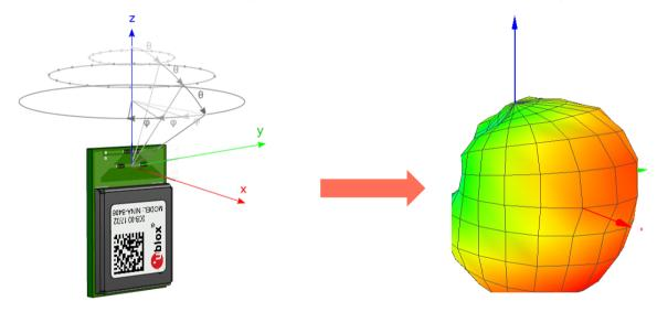
Figure 5: Measurement procedure for determining radiation patterns
