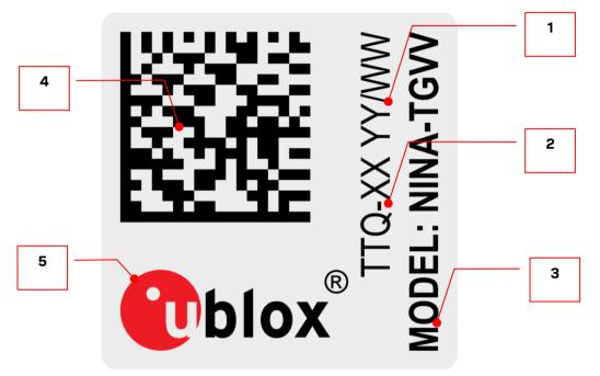
Figure 13: Layout of the NINA-B50 module label
