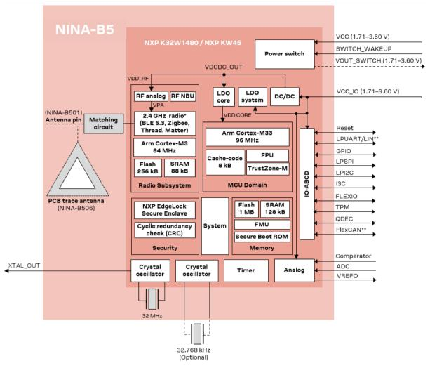
\* IEEE 802.15.4 (Thread<sup>®</sup>, Matter<sup>™</sup>, and Zigbee<sup>™</sup>) is only supported by NINA-B50 professional grade modules. \*\* FlexCAN and LIN bus are only supported by NINA-B50 automotive grade modules.
