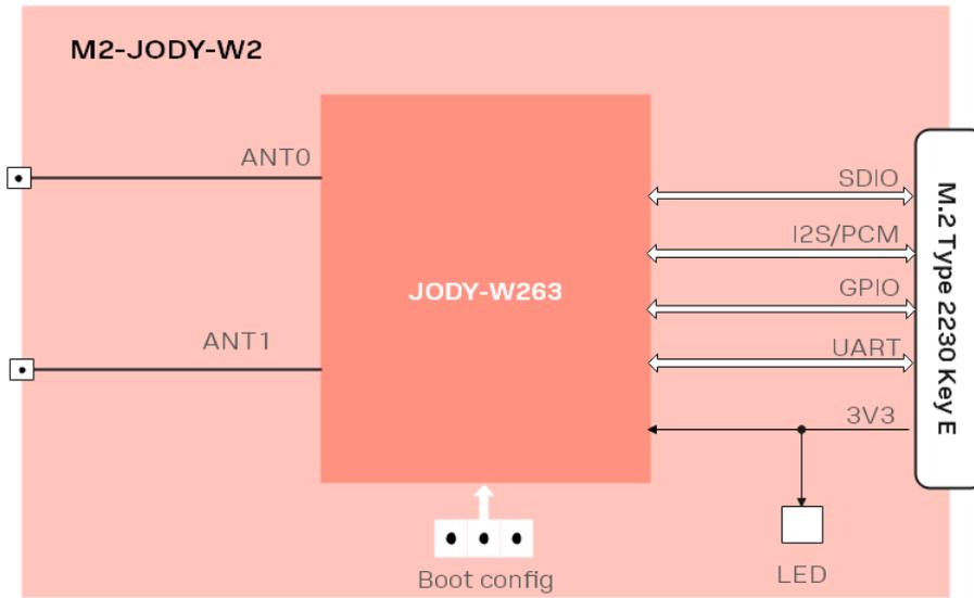
Figure 1: Block diagram of the M2-JODY-W2 card module
