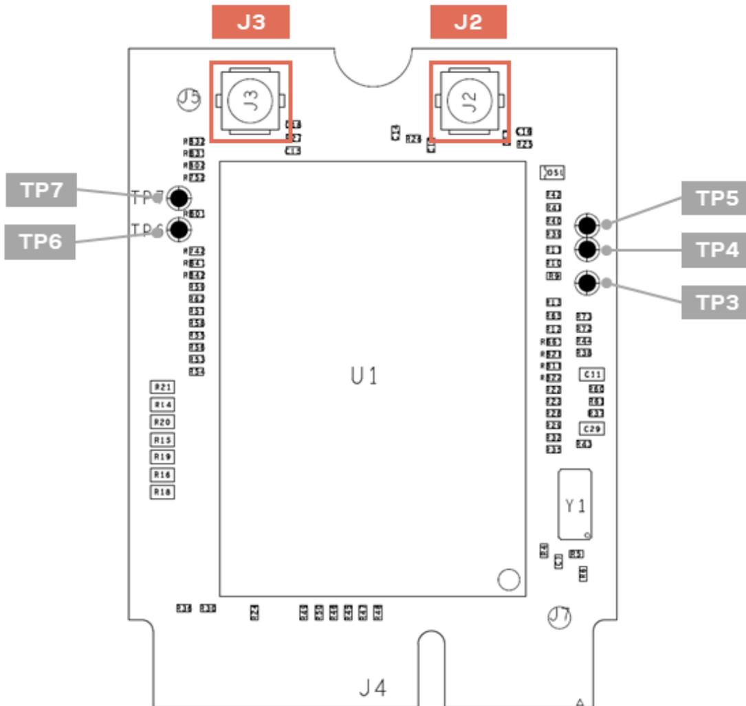
Figure 5: Location of M2-JODY-W2 antenna U.FL connectors
