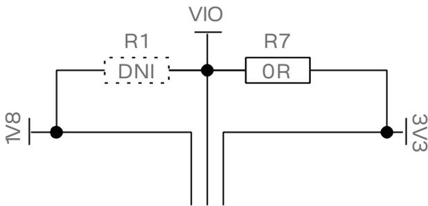
Figure 6: Placement of 0 Ω resistor to change VIO from 1V8 V to 3V3
