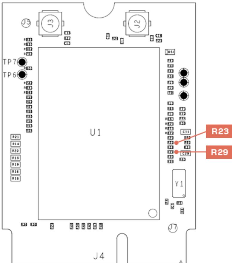
Figure 3: Position of resistors R23 and R29 on M2-JODY-W2 (top side)
