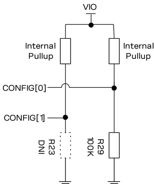
**Figure 2: Default configuration of the M2-JODY-W2 boot pins**
