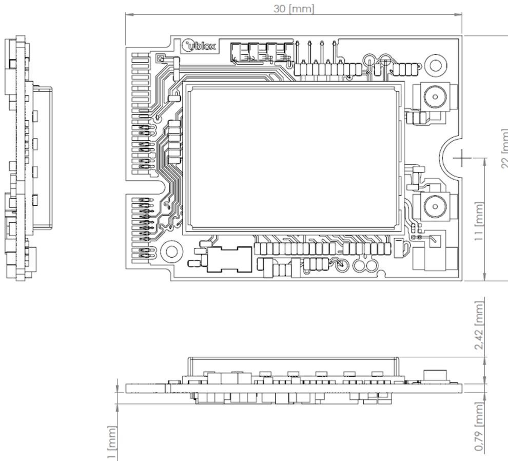
Figure 10: Physical dimensions of the M2-JODY-W2 card
