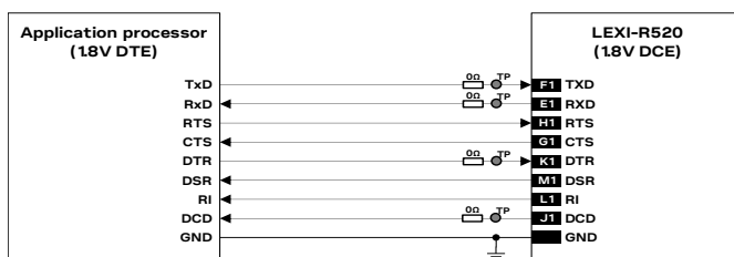
Figure 48: 1 UART interface application circuit with complete V.24 link in DTE/DCE serial communication (1.8 V DTE)
