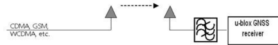
Figure 20: Measures against in-band interference
