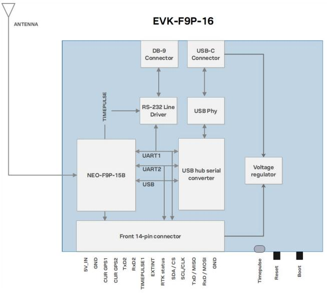
Figure 12: EVB-F9P block diagram
