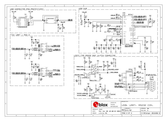
Figure 16: Schematic EVK-F9P: Connectors
