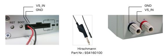
Figure 4: Example 5V DC power supply
