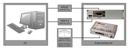
Figure 1: Connecting the unit for power supply and communication.
