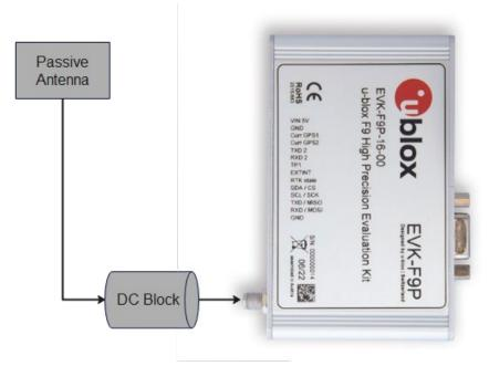
in the RF path while using passive antenna
