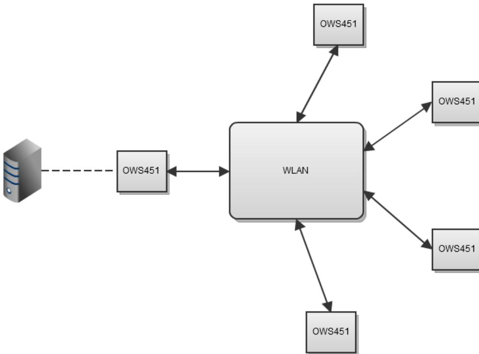
The serial port adapter on the right could be connected to some form of sensors transmitting data, which is then forwarded by the serial port adapter on the left side to the computer that monitors the process.
