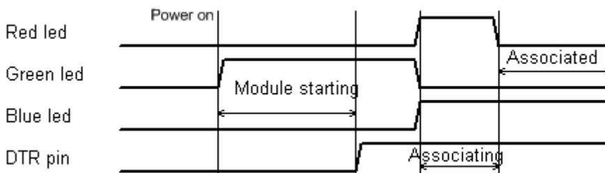
**Figure 1** Default configuration, DTR mode = at startup
