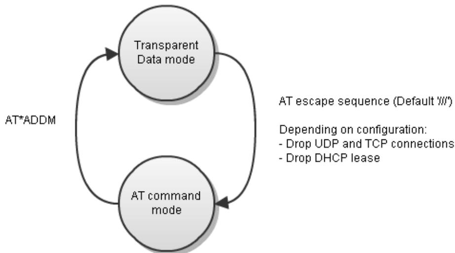
Any connection that you have with the serial port adapter module, be it serial, TCP or UDP can be used to enter AT mode. The procedure is the same as described above.
