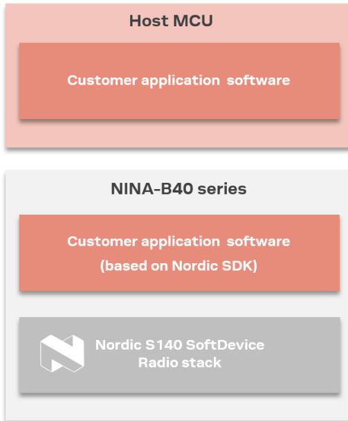
Figure 2: NINA-B40 software structure and available software options
