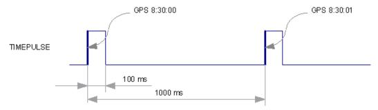
Figure 19: Time pulse signal with the example parameters
