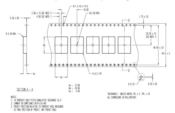
Figure 41: NEO-M9L tape dimensions (mm)
