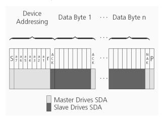
Figure 13: I2C current address read access
