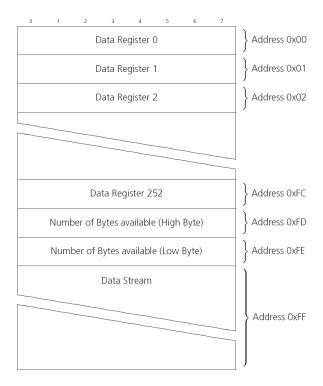
Figure 11: I2C register layout
