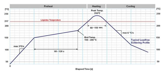
Figure 39: Soldering profile for automotive grade NEO-M9L
