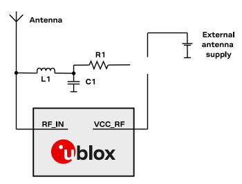
Figure 31: NEO-M9L active antenna example circuit (bias-T)
