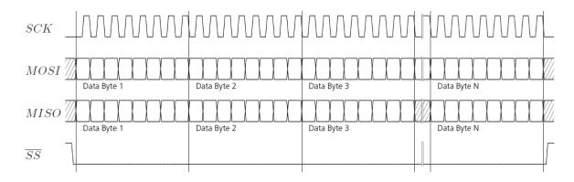
Figure 15: SPI back-to-back read/write access
