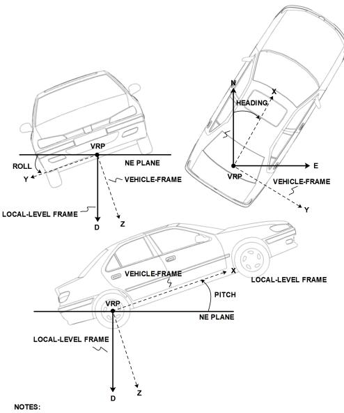
N = NORTH, E = EAST, D = DOWN, IMU-FRAME ALIGNED WITH VEHICLE-FRAME
