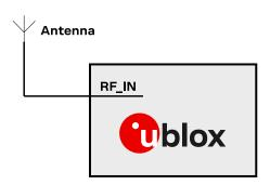
Figure 30: Passive antenna example circuit
