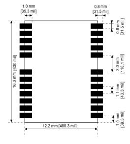
Figure 34: NEO-M9L suggested footprint (i.e. copper mask)
