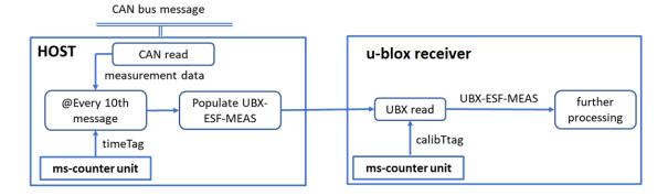
Figure 43: Example of odometer data transfer and processing
