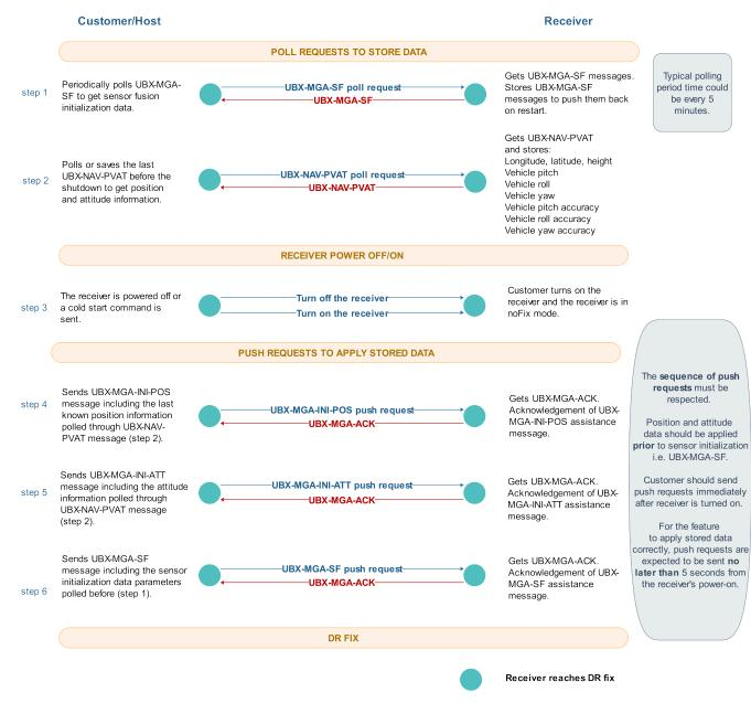
Figure 8: Advanced calibration handling operational steps
