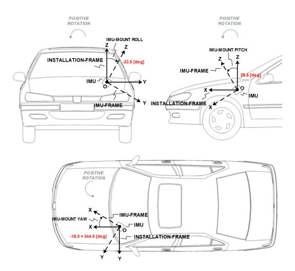
Figure 3: Installation frame
