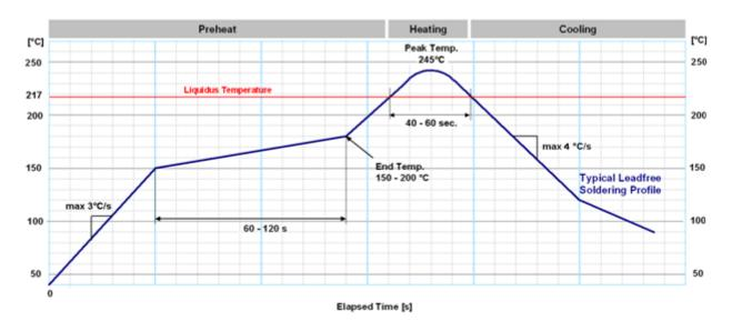
Figure 38: Soldering profile for professional grade NEO-M9L
