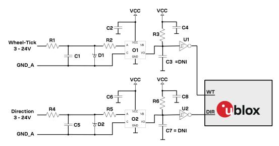
Figure 29: Example WT and DIR design
