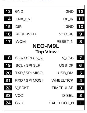
Figure 26: NEO-M9L pin assignment
