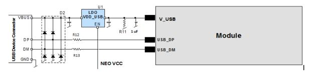
Figure 16: NEO-M9L example circuit for USB interface
