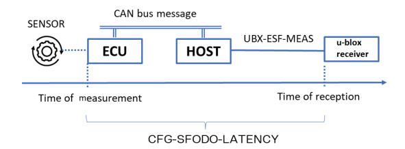
Figure 42: Example of odometer measurement data path
