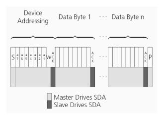
Figure 14: I2C write access
