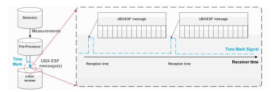
Figure 5: Time mark on external input
