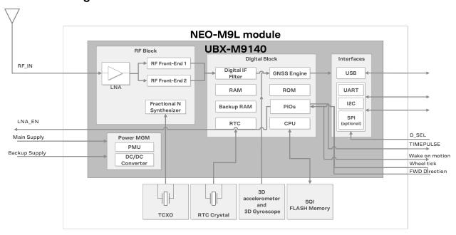
Figure 1: NEO-M9L block diagram
