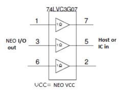
Figure 9: NEO-M9L output isolation
