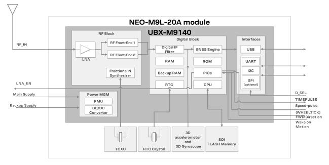
Figure 1: NEO-M9L-20A block diagram
