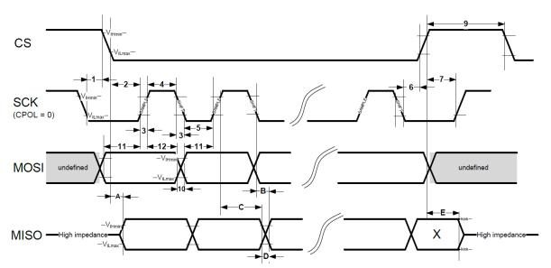
Figure 3: NEO-M9L-20A SPI specification mode 1: CPHA=0 SCK = 5.33 MHz
