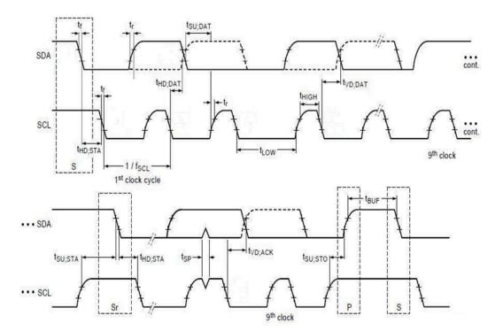
Figure 4: NEO-M9L-20A I2C slave specification
