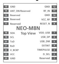
Figure 2: Pin Assignment
