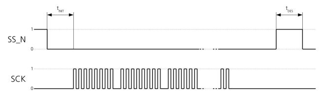
Figure 3: SPI timing diagram
