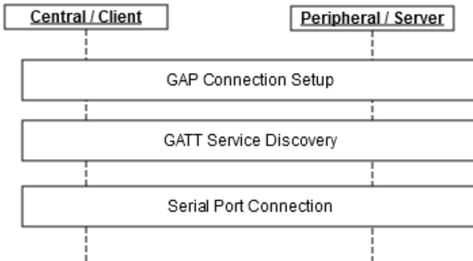
Figure 1: SPS connection setup
