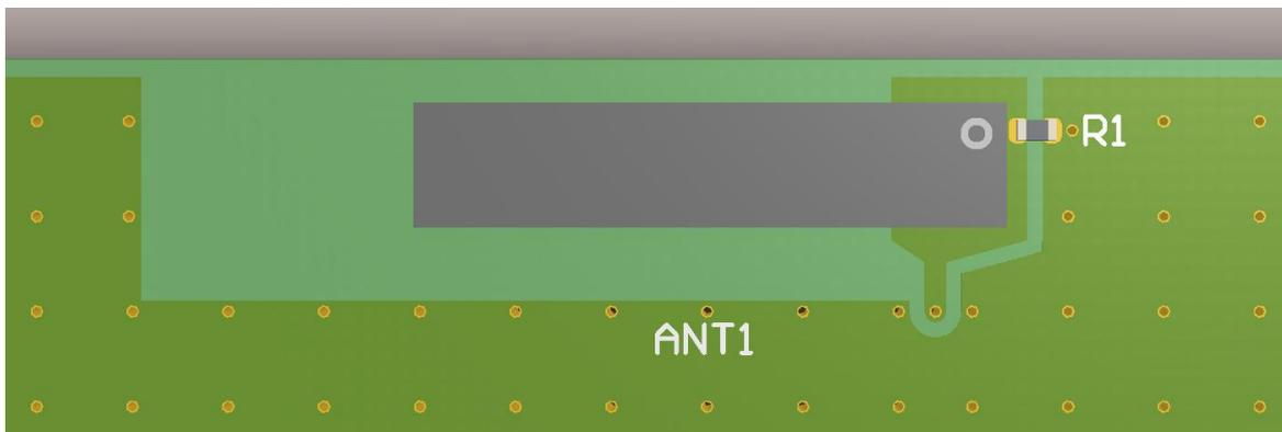
**Figure 9:** Antenna goes to a via and the matching components are placed on the backside. The via should be designed such that it makes a good  $50\ \Omega$  transition to the backside.
