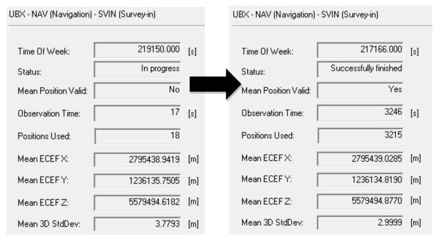
Figure 4: Base Station moving from Survey-in Mode to Fixed Mode
