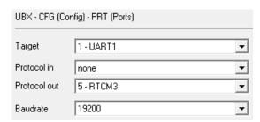
Figure 7: Configuring Base radio link
