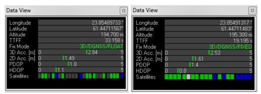
Figure 21: Data View shows "FLOAT" or "FIXED" on Rover
