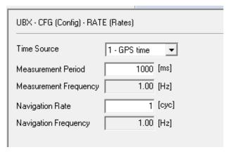
Figure 13: Navigation rate set to 1 Hz
