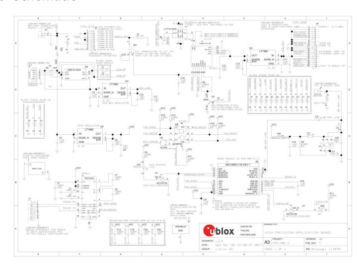
Figure 29: Schematics of C94-M8P-E application board
