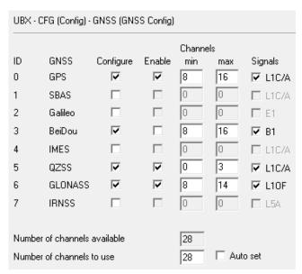
Figure 1: Configuration of the NEO-M8P-2 GNSS module on C94-M8P application board
