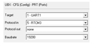
Figure 8: Configuring Rover radio link
