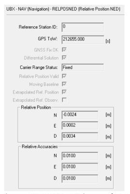
Figure 22: UBX-NAV-RELPOSNED in u-center for Rover
