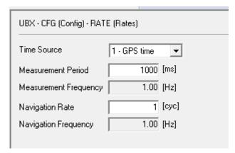
Figure 16: Configuring Navigation rate
