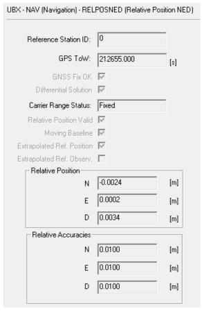
Figure 19: UBX-NAV-RELPOSNED in u-center for Rover
