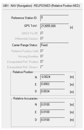
Figure 25: UBX-NAV-RELPOSNED showing flags Extrapolated Ref Position and Extrapolated Ref Observation
