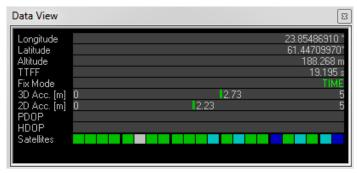
Figure 17: Data View shows "TIME" when Base is in FIXED mode
