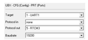
Figure 12: Configuring Base radio link
