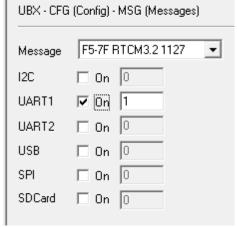
Figure 11 For a GPS+BeiDou setup, enable the RTCM messages 4072, 1077, 1127 on UART1 port
