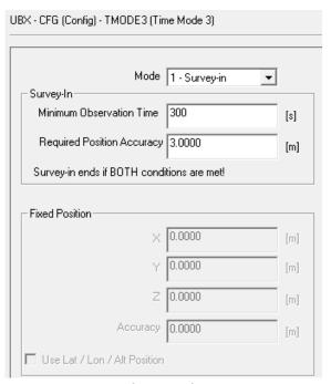
Figure 3: Survey-in configuration for a Base Station
