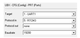
Figure 15: Configuring Rover UART port
