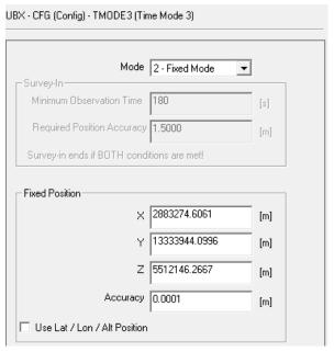
Figure 2: Fixed Position Mode configuration for a Base Station
