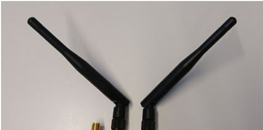
Figure 2: Example of orthogonally polarized dipole antennas
